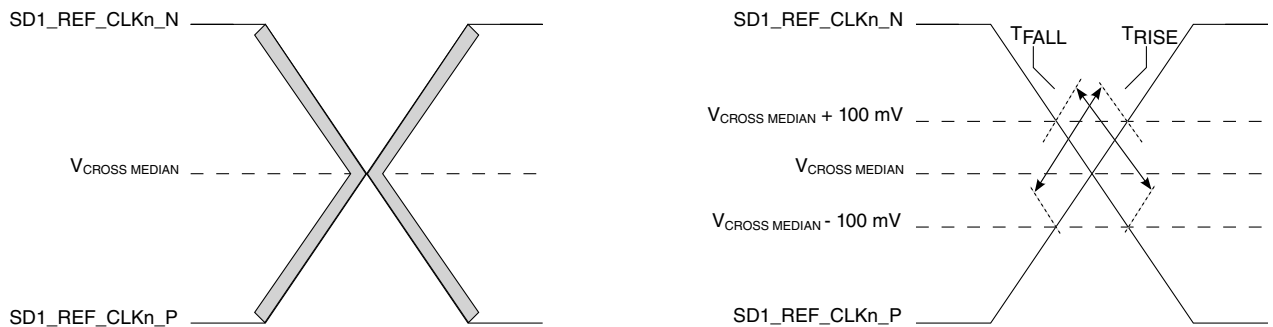
Figure 80. Single-ended measurement points for rise and fall time matching
